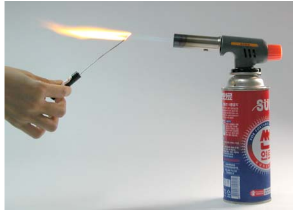
Fig. 4. The picture of putting a nichrome wire stained with NaCl into the torch flame
